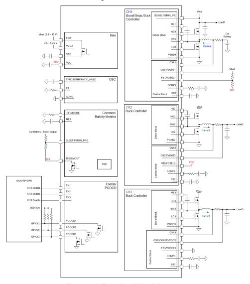
Figure 1-1. Functional Block Diagram
