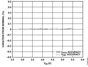
Figure 3. Boost Regulator Line Regulation,  $V_{POS} = 15 V$ , Switching Frequency  $(f_{SW}) = 1.2 \text{ MHz}$ , 15 mA Load,  $T_A = 25 ^{\circ}\text{C}$
