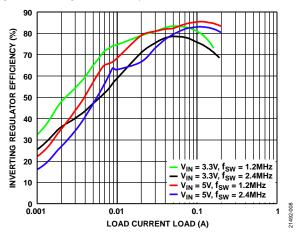
Figure 8. Inverting Regulator Efficiency vs. Load Current,  $V_{NEG} = -15 V$ ,  $T_A = 25$ °C
