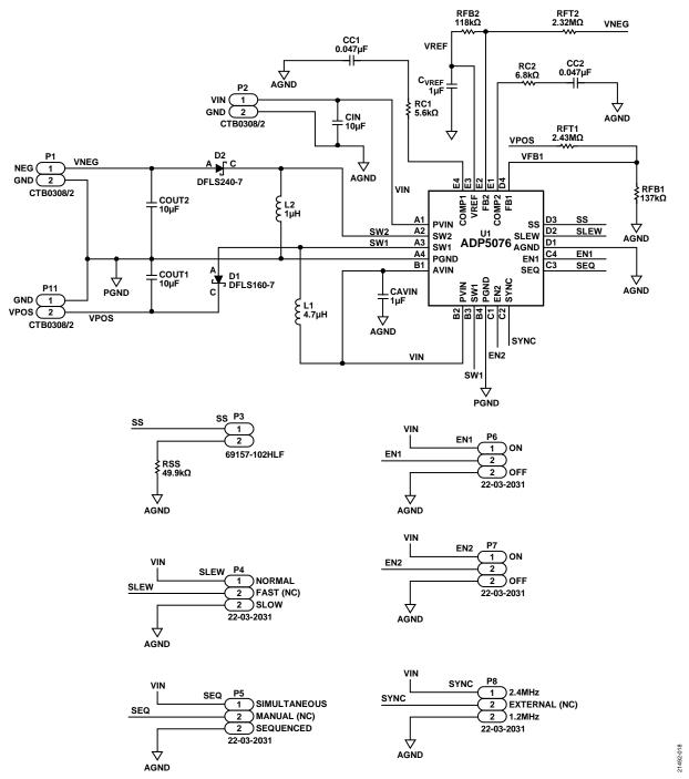
Figure 9. Evaluation Board Schematic for the ADP5076CB-EVALZ
