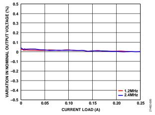
Figure 5. Boost Regulator Load Regulation, Input Supply Voltage Range  $(V_{IN}) = 5 V$ ,  $V_{POS} = 15 V$
